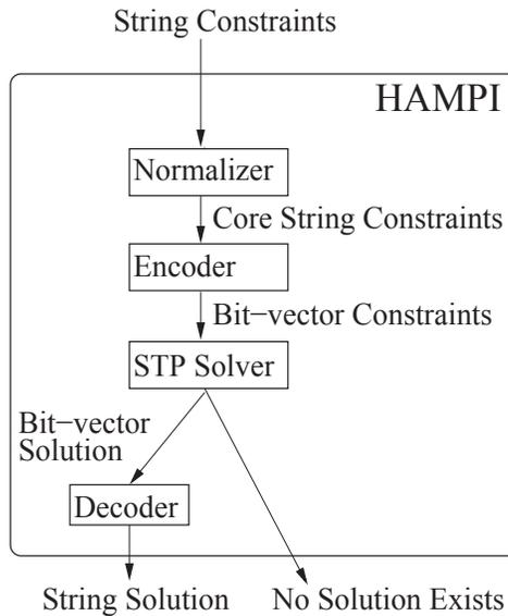
Fig. 3. Schematic view of the HAMPI string constraint solver. Input enters at the top, and output exits at the bottom. Section 3 describes the HAMPI solver.
