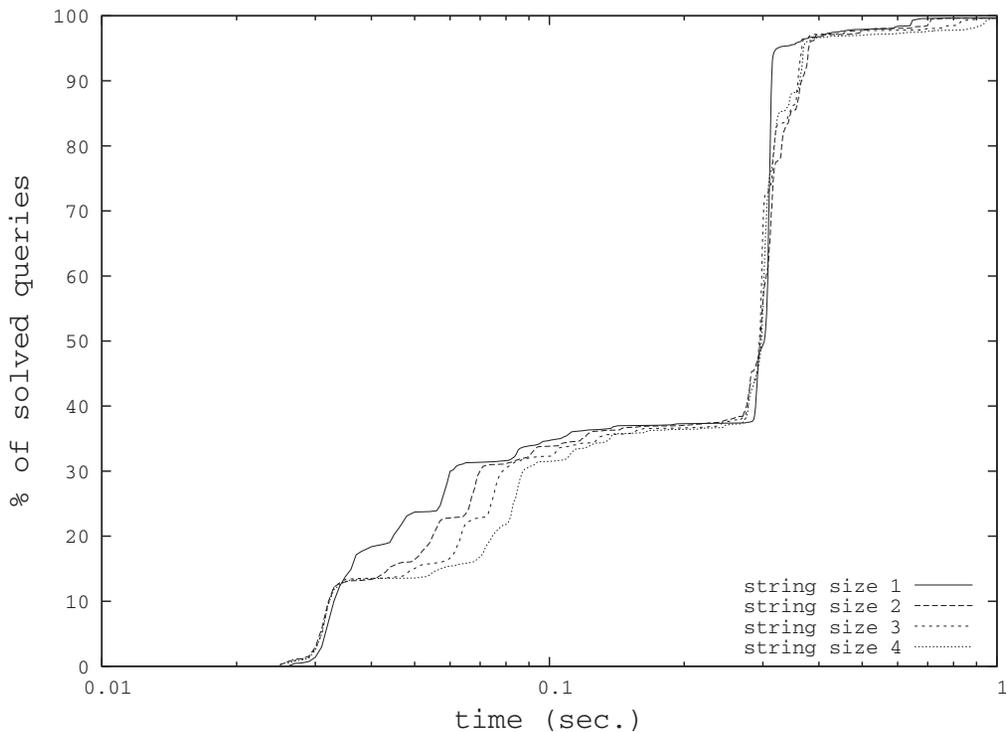
Fig. 9. Percentage of queries solvable by HAMPI, in a given amount of time, on data from Wassermann and Su [2007]. Each line represents a distribution for a different size of the string variable. All lines reach 99.7% at 1 second and 100% before 160 seconds. Section 5.1 describes the experiment.
